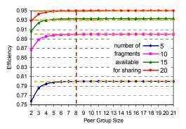
Figure 2. Effect of Peer Group Size on the Efficiency of Fragment Exchange
