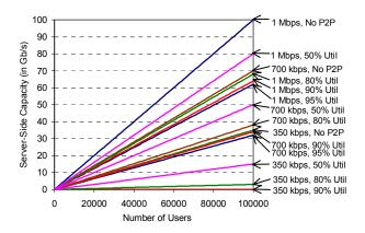
Figure 1. Benefits of using a well-designed peer-to-peer solution (Assumption: Peer Upload Capacity is 400 Kbps)
